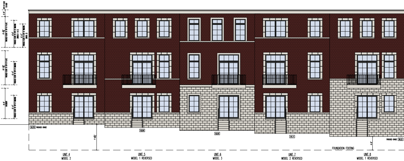
UNITS 4-8: SOUTH ELEVATION (MLK Jr DRIVE) SCALE: 1/4" = 1'-0"
