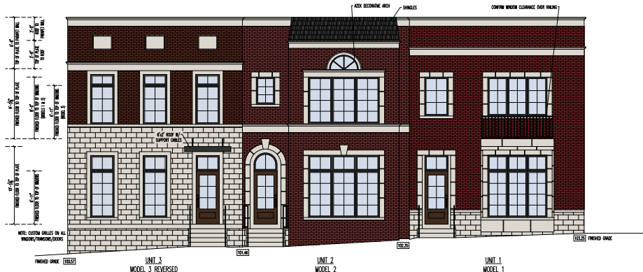
UNIT 3 MODEL 3 REVERSED UNIT 2 MODEL 2 UNIT 1 MODEL 1 UNITS 1-3: NORTH ELEVATION (MOSS AVENUE) SCALE: 1/4" = 1'-0"
