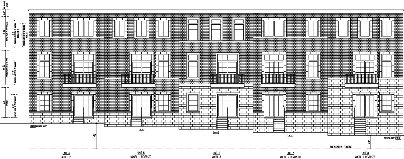
UNITS 4-8: SOUTH ELEVATION (MLK Jr DRIVE) SCALE: 1/4" = 1'-0"
