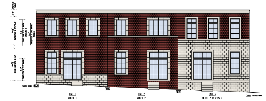
UNITS 1-3: SOUTH ELEVATION (FACING PARKING LOT) SCALE: 1/4" = 1'-0"
