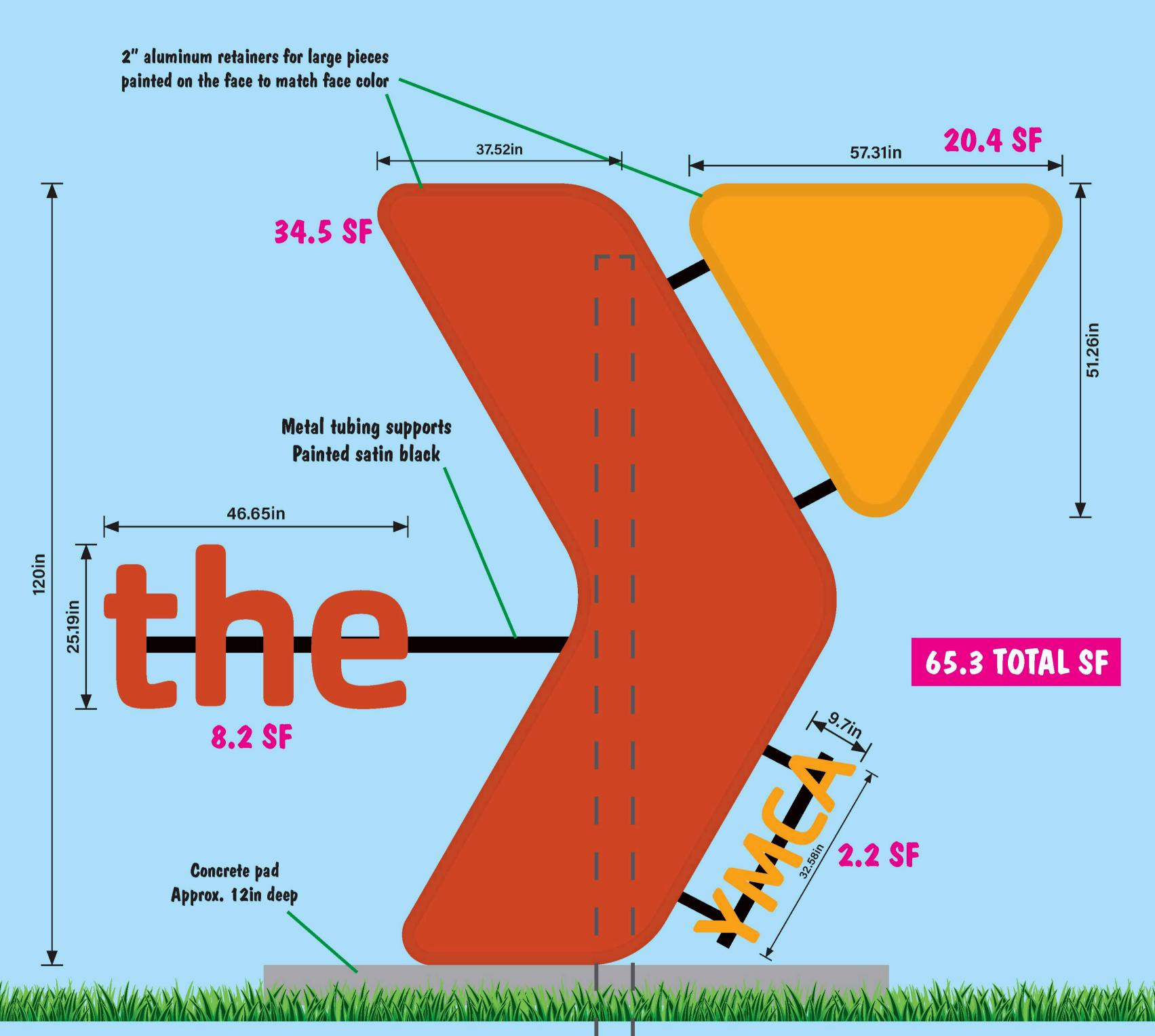
6x6 1/4in wall square steel support pole Runs up the center of the sign
