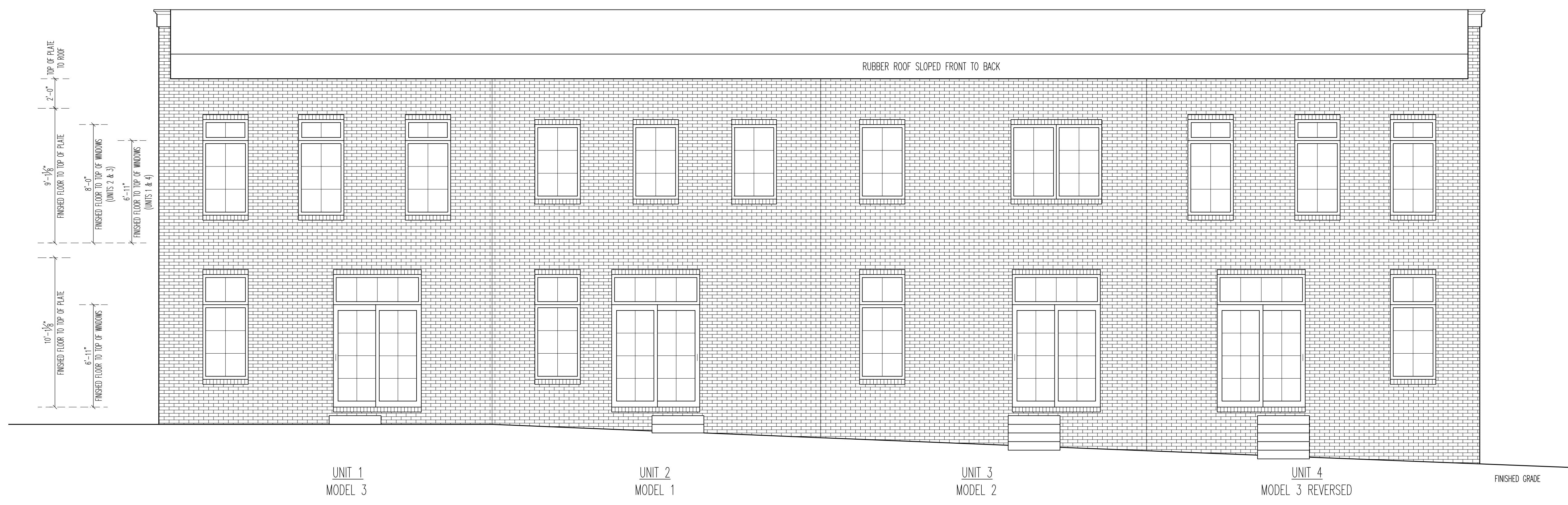
UNITS 1-4: SOUTH ELEVATION (FACING PARKING LOT) SCALE: 1/4" = 1'-0"
