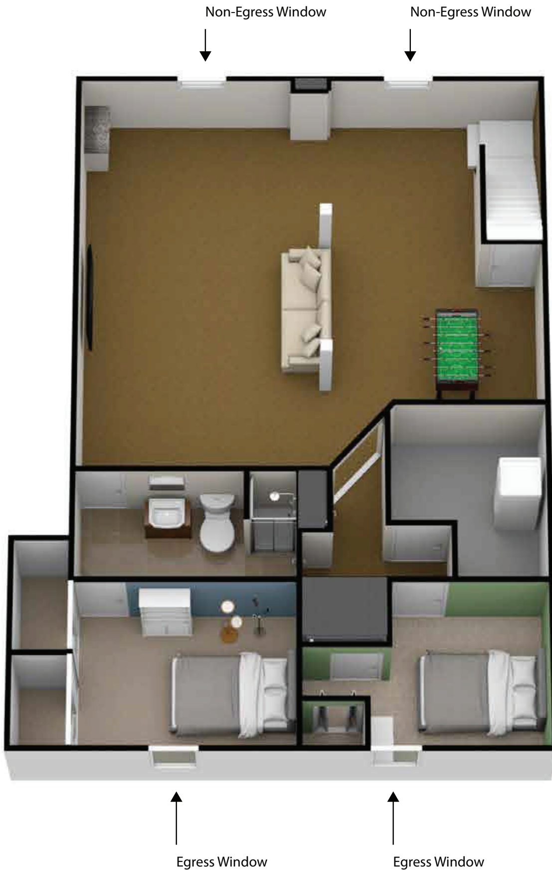
Site Plan: Basement Egress (and Non)
